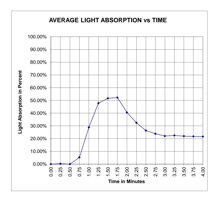
MODIFIED ASTM D635 TESTING
